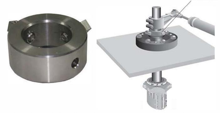
Tides Marine Rudder Collars are for use on power boats. Machined from 304 stainless steel, each unit comes with two threaded locking screws. A third "indexed hole" (which is not threaded) is machined into each Rudder Collar and may be used as a guide to drill "dimples" in the rudder stock. Simply measure your rudder stock diameter (.000") and select the matching part number below.
