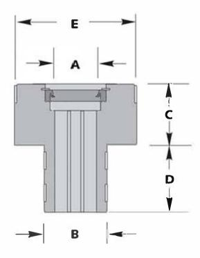
To determine which part to order, measure the exact diameter of the rudder stock (.000") and the O.D. of the bronze rudder port to which the unit will be connected. Note your combination of rudder stock diameter and rudder port O.D. in the table below. Confirm that there is sufficient space to accommodate the flange height and the barrel height plus 1" of space between the Type I unit and the rudder port. Finally, confirm that there is clearance for the O.D. of the Type I assembly.
