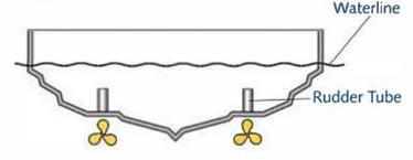
Type 2: Molds which require modification to achieve a "flat" surface or pocket for mounting a standard flange-type liner.
