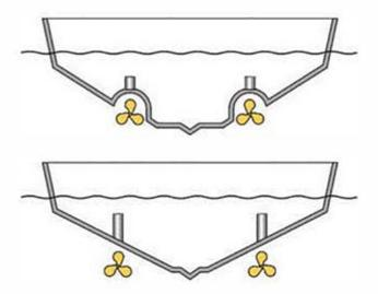
Type 3: Molds which require modification to accept an angled liner to match dead rise and rocker angles.
