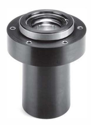
The Tides Marine Type C rudder port is used in vessels constructed of FRP, steel or aluminum which have an integral rudder port tube and flange. Unlike the typical assemble with separate bearing and packing, the Type C unit combines both sealing and bearing functions in a cost-effective housing. It is an ABS- and Lloyds-approved design and offers a substantial "bearing surface" to "rudder stock diameter" ratio.
