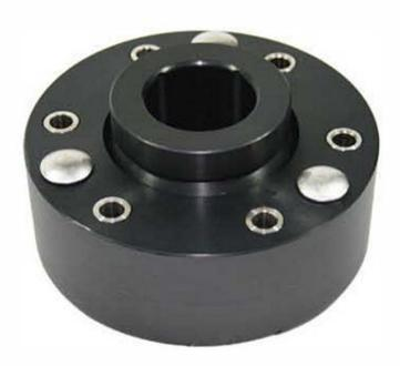
The TidesMarine Upper Rudder Bearing-Standard (URB-STD) is designed to be mounted directly on top of the rudder shelf. It is an ABS- and Lloyds-approved, self-aligning design which accommodates up to 10 degrees of off-axis alignment between the mounting surface (rudder shelf) and the rudder stock. As a result, it requires no shimming during installation and won't load the rudder shaft during vessel operation.
