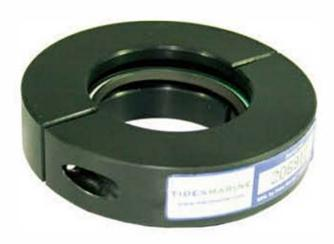
Tides Marine Spare Rudder Seal Carriers were developed as a convenient place to store spare lip seals on the rudder stock. The unit also makes the job of replacing the lip seal in a Tides Marine rudder port easier and is recommended as an accessory for all Tides Marine rudder ports. Installed at the same time as the RPB, they allow the lip seal to be replaced without uncoupling the rudder stock from the steering system or dropping the rudder.
