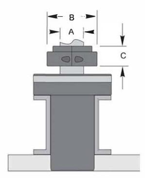
Measure the exact diameter (.000) of your rudder stock. Next, confirm that there is sufficient space to accommodate both the diameter of the Carrier (Column "B" in the table below) and its the overall height (Column "C" in the table below).
